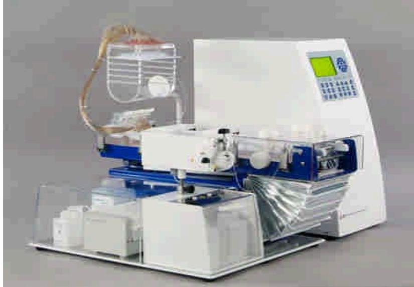
The BD Free Flow Electrophoresis System (FFE) is a new product used for semi-preparative fractionation and enrichment of protein or cellular samples. The electrophoresis works in a thin film of aqueous liquids in the absence of any kinds of stationary phases like gels. It's capable of separating simple or complex protein samples. It's compatible with most downstream separation technologies.
